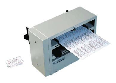
12up business card slitter easily converts 8 1/2" x 11" sheets to finished 2" x 3 1/2" business cards with a simple two pass operation. Premium features include perfect cuts, catch tray, receptacle and adjustable feed to accommodate different types of material thickness. This unit does not accommodate bleed printing.
